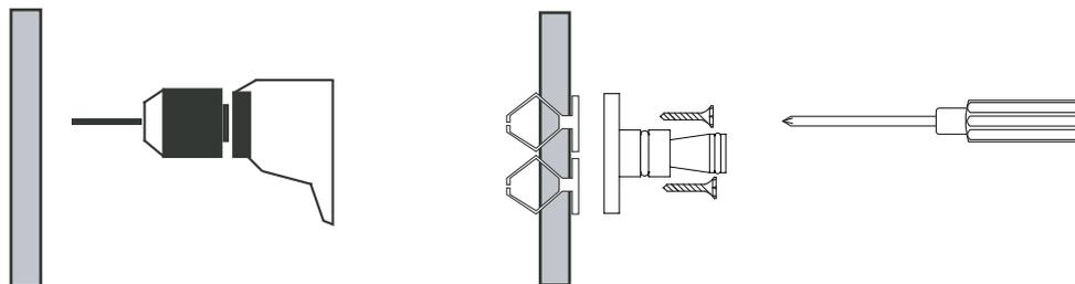
Mark the two screw hole positions by using the mounting hardware post. Using a drill, pre-drill holes for the toggles. Fold the toggle's legs and insert them into the wall. The mounting hardware posts can be secured by screwing the screws into the toggles.
