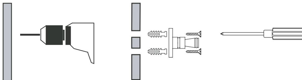
Measure the dimensions carefully. Mark the two screw hole positions by using the mounting hardware post. Using a drill, pre-drill the holes. Insert anchors into the wall. Secure the mounting hardware posts by screwing the screws into the anchors.
