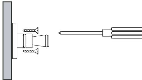
For wooden surface, the mounting hardware posts can be secured by screwing the screws directly into the wall.
