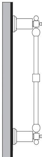
Adjust the bar posts if necessary and secure by firmly tightening the set screws with the allen key.
