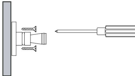
For wooden surfaces, the mounting hardware posts can be secured by screwing the screws directly into the wall.
