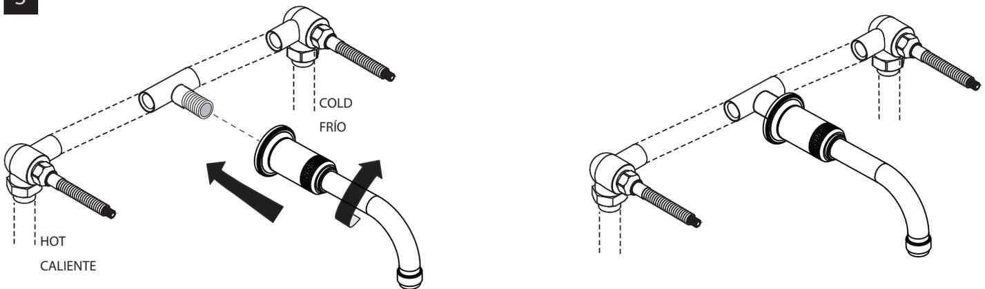
Note: The length of threaded pipe coming out from the finish wall should be no longer than 1/2".
