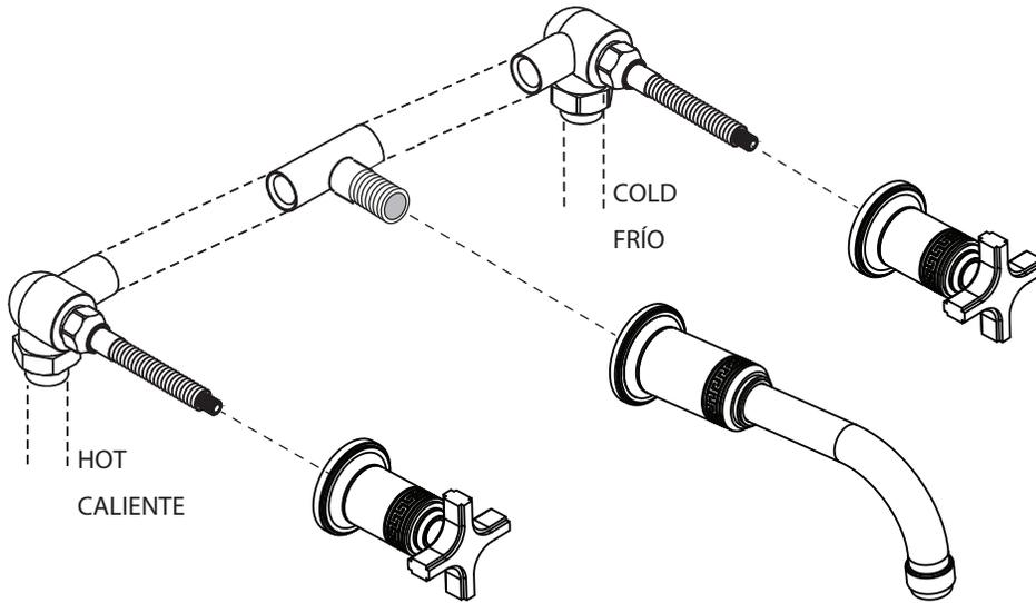
Using 1/2" IPS, connect corner valves to the spout base at the desired spread.
